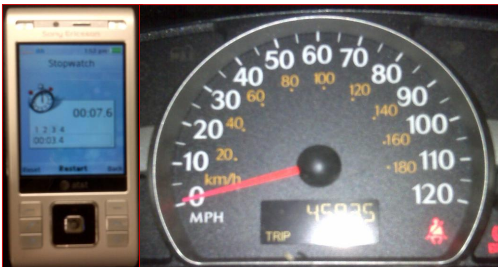
Figure 3: Stopwatch and analog speedometer used to determine the rate of deceleration.
