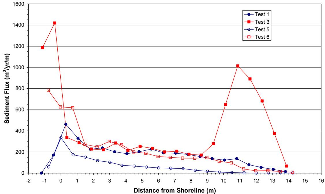
Fig. 7. Cross-shore distribution of measured longshore sediment transport
