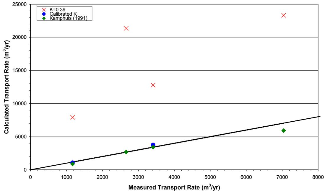
Fig. 6. Comparison of calculated to measured transport rates
