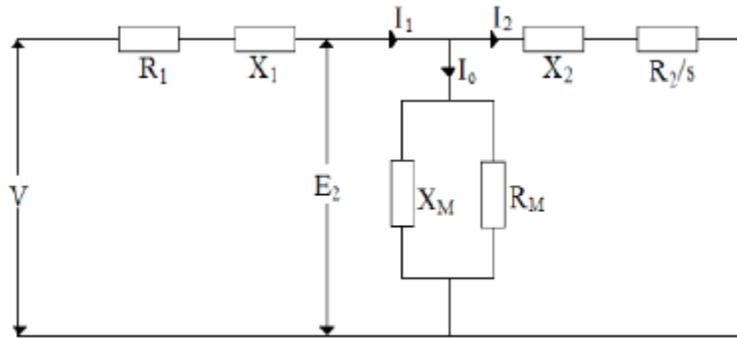
Figure 2.1 Equivalent circuit of IM [9]
