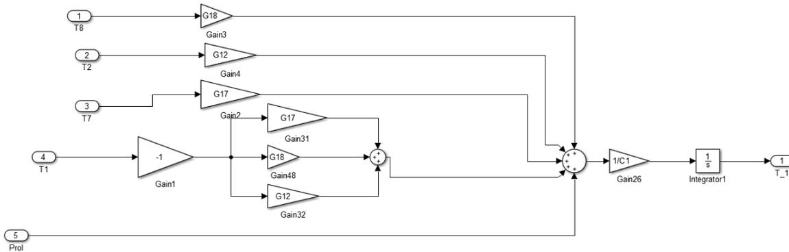
Figure 4.4 Example of temperature calculation in rotor bars
