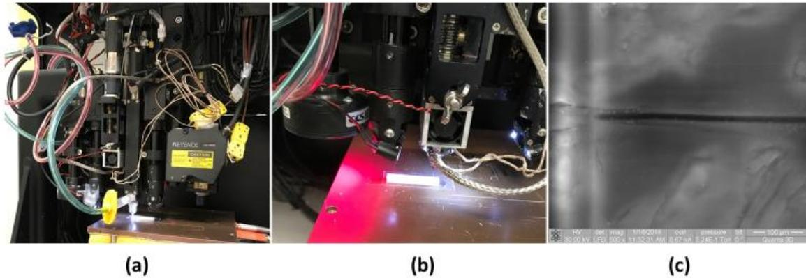
**Figure 4.** DPAM process to print an optical fiber onto a surface. (a) Urethane Cladding being dispensed onto an ABS form, (b) The PMMA core is printed onto the surface, and (c) The fiber embedded into a channel on the surface of the urethane cladding material.
