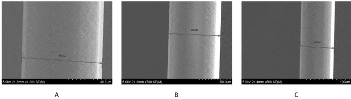
**Figure 11.** SEM image of the variation in diameter due non-uniform traverse speed across the extrusion span. (a) The nominal diameter of about 77  $\mu\text{m}$  is achieved from a 50  $\mu\text{m}$  nozzle, (b) The max diameter observed is about 85  $\mu\text{m}$  at the start of the extrusion, and (c) Once the extruder reaches target traverse speed the thickness is down to the nominal 77  $\mu\text{m}$ .
