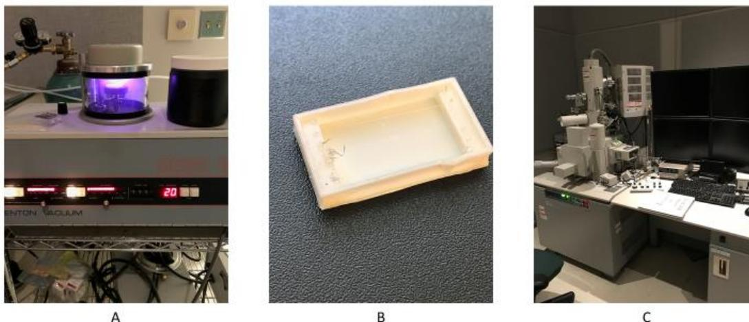
**Figure 8.** Sample preparation for SEM. (a) Sputter of a gold/palladium coating onto a PMMA plastic fiber so it is conductive, (b) Sample fiber after sputter coating, and (c) Actual SEM equipment used in imaging of fiber.
