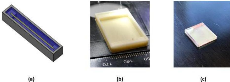
**Figure 3.** DPAM optical fiber design. (a) Concept of DPAM optical interconnect with an ABS housing, a PMMA core and an UV curing adhesive cladding, (b) Packed cores after printing, and (c) Finished 10 core interconnect with cladding and end facets prepared for testing.
