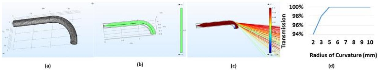
**Figure 1.** Numerical simulation of optical interconnect using COMSOL ray tracing. (a) 50-micron fiber was modeled, (b) Rays of light were injected into the fiber, (c) Decreasing bend radii were evaluated until a critical angle was reached and light escapes the fiber, and (d) Numerical simulation predicts high transmission levels at small angles of less than 3 to 5  $\mu\text{m}$ .
