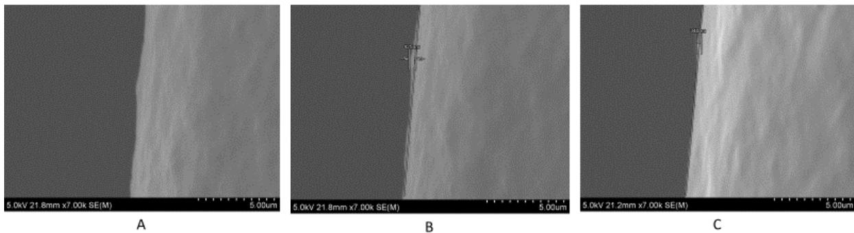
**Figure 10.** SEM results indicated a smooth optical core. (a) Average surface variation is very small, (b) The maximum surface variation measured is less than 425 nm., and (c) The average surface roughness is much closer to 340 nm.
