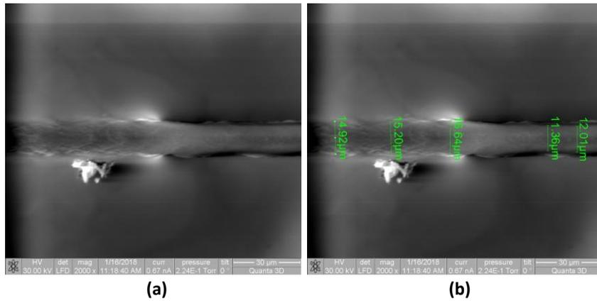
**Figure 13.** Single mode fiber printed on a cladding surface and embedded in a cladded surface. (a) FDM parameters can either imbedded in the fiber core in the cladding or in channel on the surface, and (b) Quality of fiber printed in a channel on the cladding appear much smoother and with a more uniform diameter.
