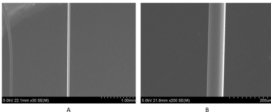
**Figure 9.** SEM images of smooth straight PMMA fibers that were produced using the DPAM process. (a) A 30x view of the fiber that indicates how straight the fiber has been extruded, (b) A 200x view of the fiber showing a very smooth surface.
