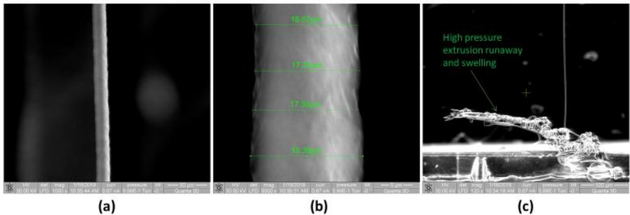
**Figure 12.** SEM evaluation of DPAM optical waveguide with a 9  $\mu\text{m}$  FDM tip. (a) Typical surface of a DPAM manufactured PMMA fiber, (b) Surface roughness of between 1 and 2  $\mu\text{m}$  is measured, and (c) Control of fiber during the FDM process is difficult with high pressure and temperatures required and leads to swelling and runaway extrusion.
