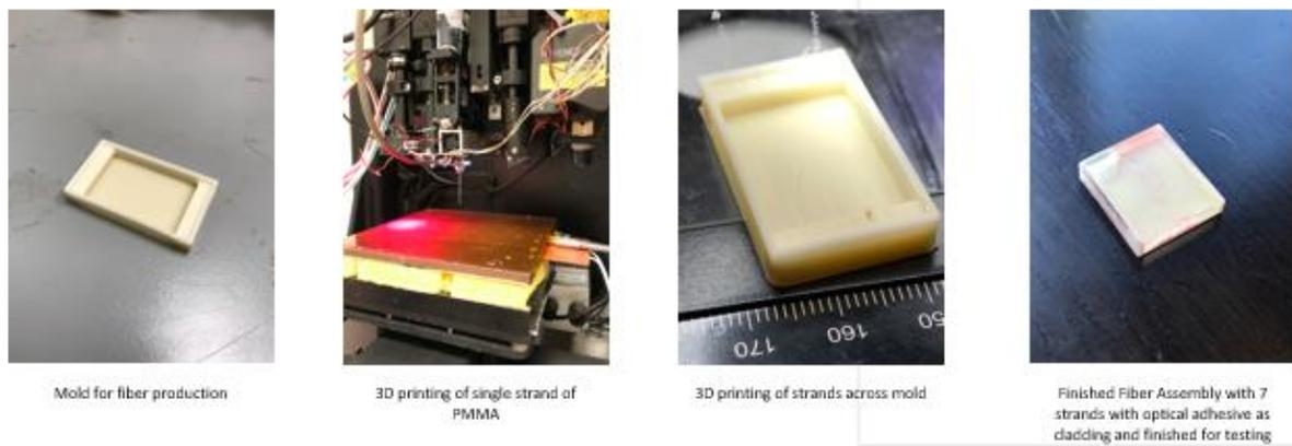
**Figure 2.** Fabrication of optical interconnects. (a) A guided channel base cladding, (b) FDM printing of a filament, (c) Multiple fiber printing, and (d) Finished optical assembly.
