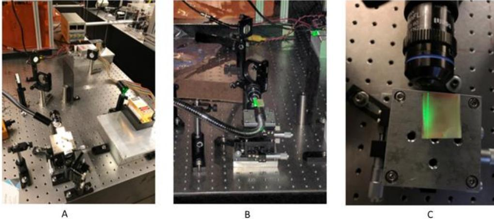
**Figure 7.** Laser evaluation of the digitally manufactured plastic optical fiber. (a) Actual laser test station setup, (b) The test sample in the rig with 532 nm wavelength laser is being used for the testing, and (c) Actual transmission of light through the fabricated plastic optical waveguide.
