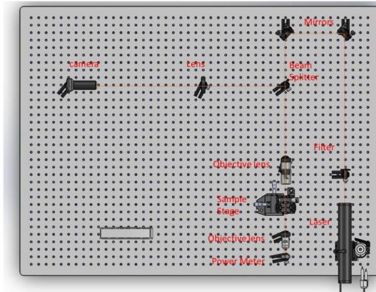
**Figure 5.** Laser test station. This setup uses a microscope objective to focus the laser and uses reflected light back through the beam splitter to see the front of the optical fiber, for aiming the laser at the center of the end facet of the fiber.
