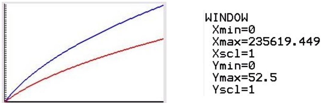
Figure 2: Comparison of a rocket trajectory on a gravitational turn with the assumption of constant gravity (blue) versus inverse square distance gravity (red).
