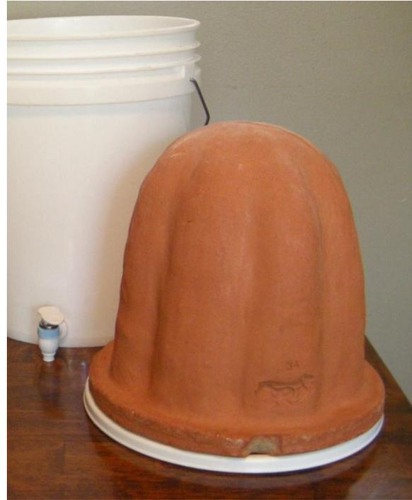
**Figure 1:** FilterPure filter sitting bottom up on a bucket lid.
