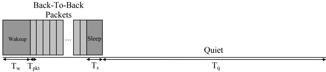
Figure 3.1 – Packet Transmission and Transitions in EEE – Best Case (not to scale)
