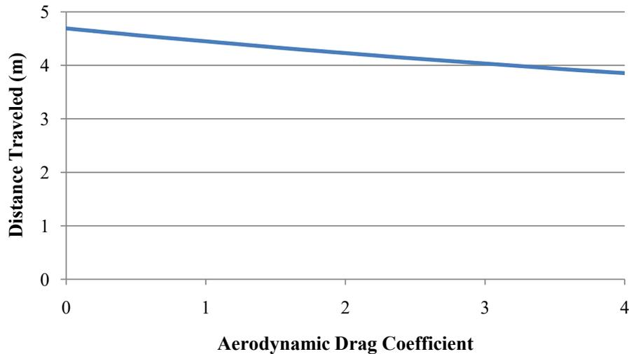
**Figure 2:** Skimboarding distance traveled by a  $29kg$  child with a surface area of  $42cm^2$ . The child enters the water at a  $2^\circ$  angle on a circular skimboard of radius  $50cm$  with initial velocity  $2.7m/s$  before reaching a terminal velocity of  $1.2 m/s$ .
