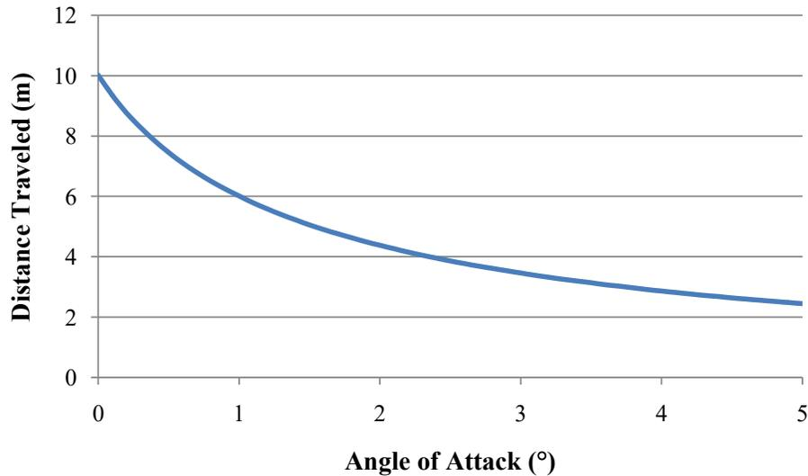
**Figure 1:** Skimboarding distance traveled by a  $29kg$  child with a surface area of  $42cm^2$ . The child enters the water on a circular skimboard of radius  $50cm$  and aerodynamic drag coefficient  $1.3$  with an initial velocity  $2.7m/s$  before reaching a terminal velocity of  $1.2 m/s$ .
