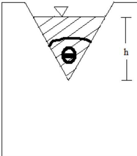
Here we have a triangular-notch weir. The inverted
