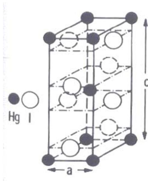
**Figure 4.1 Tetragonal Unit Cell of  $HgI_2$  [24]**
