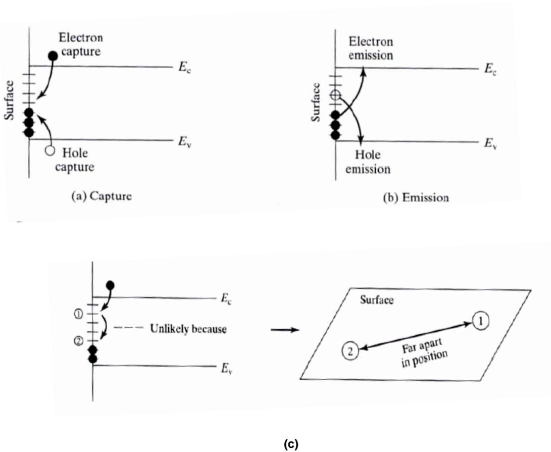
**Figure 2.7 Processes at the Semiconductor Surface**
