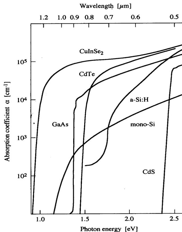
Figure 1.1: Absorption Coefficients of Various Semiconductor Materials
