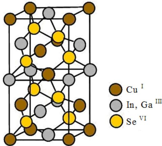
*Figure 3.1: Chalcopyrite Structure of CI(G)S*
