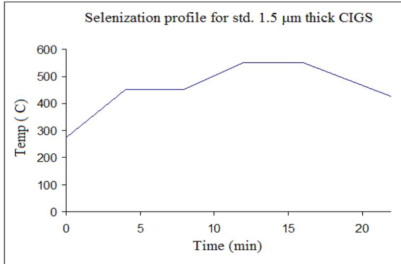
*Figure 3.4: Selenization Profile for std. 1.5μm Thick CIGS*
