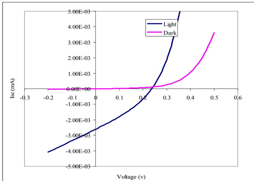
Figure 4.30: IV Curve of a 0.65µm Thick CIGS Device (C030-18)
