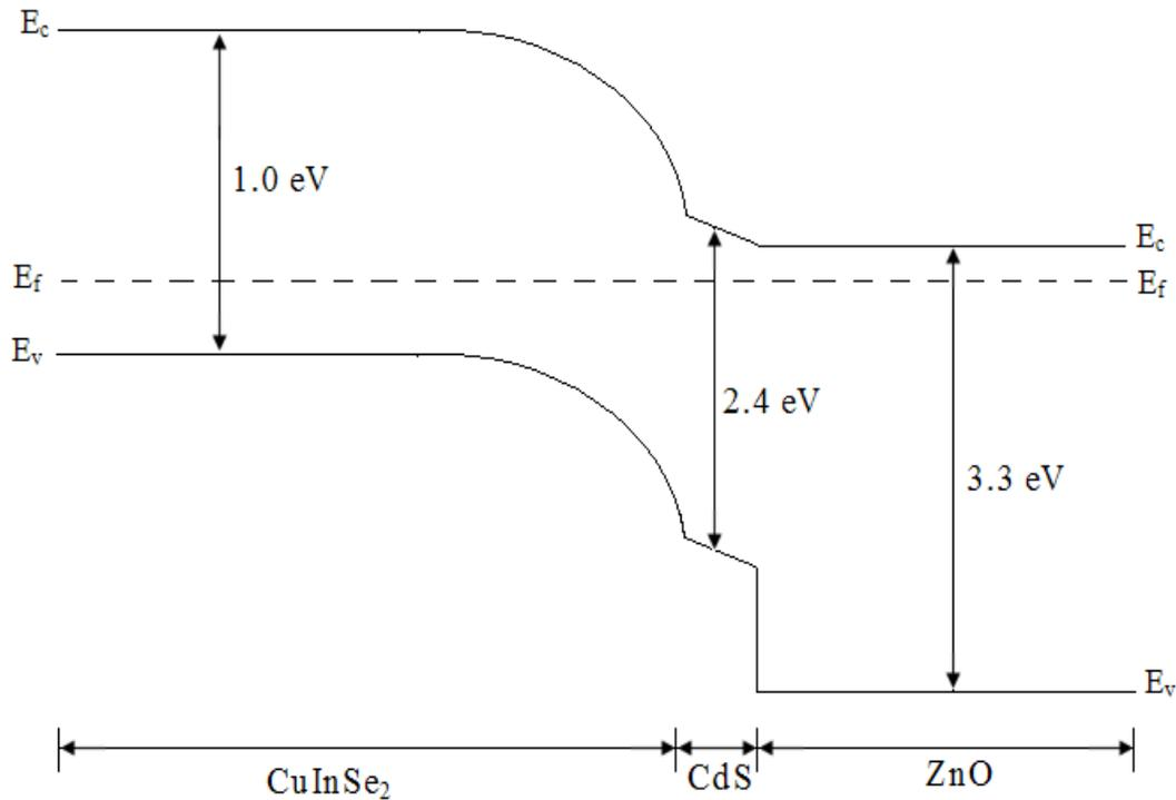
Figure 2.6: Energy-Band Diagram of a CuInSe<sub>2</sub>/CdS/ZnO Heterojunction Solar Cell
