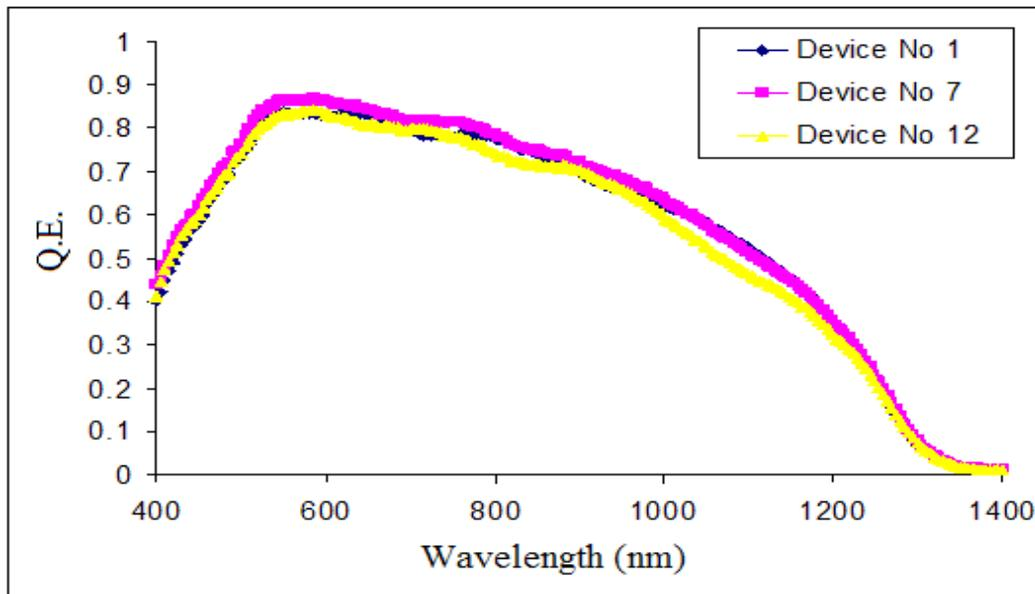
*Figure 4.9: QE Profiles of Three Devices on the Standard Run*
