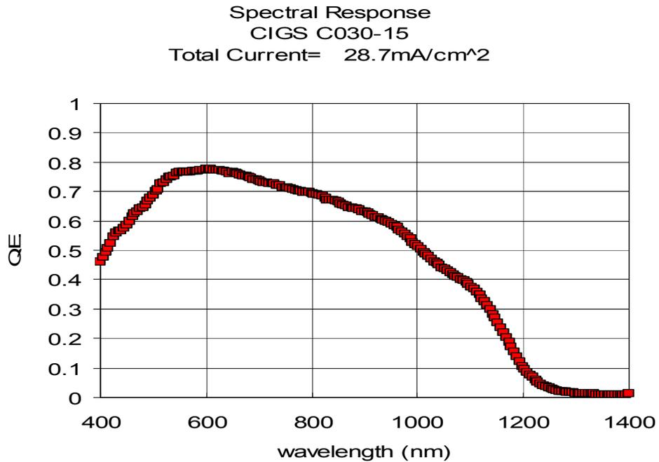
Figure 4.29: Typical Spectral Response of Devices in Run C030
