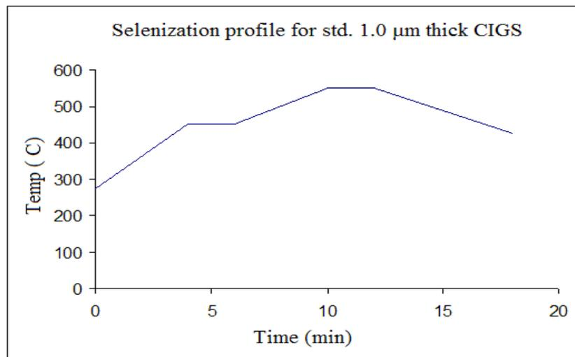
*Figure 3.5: Selenization Profile for std. 1.0μm Thick CIGS*
