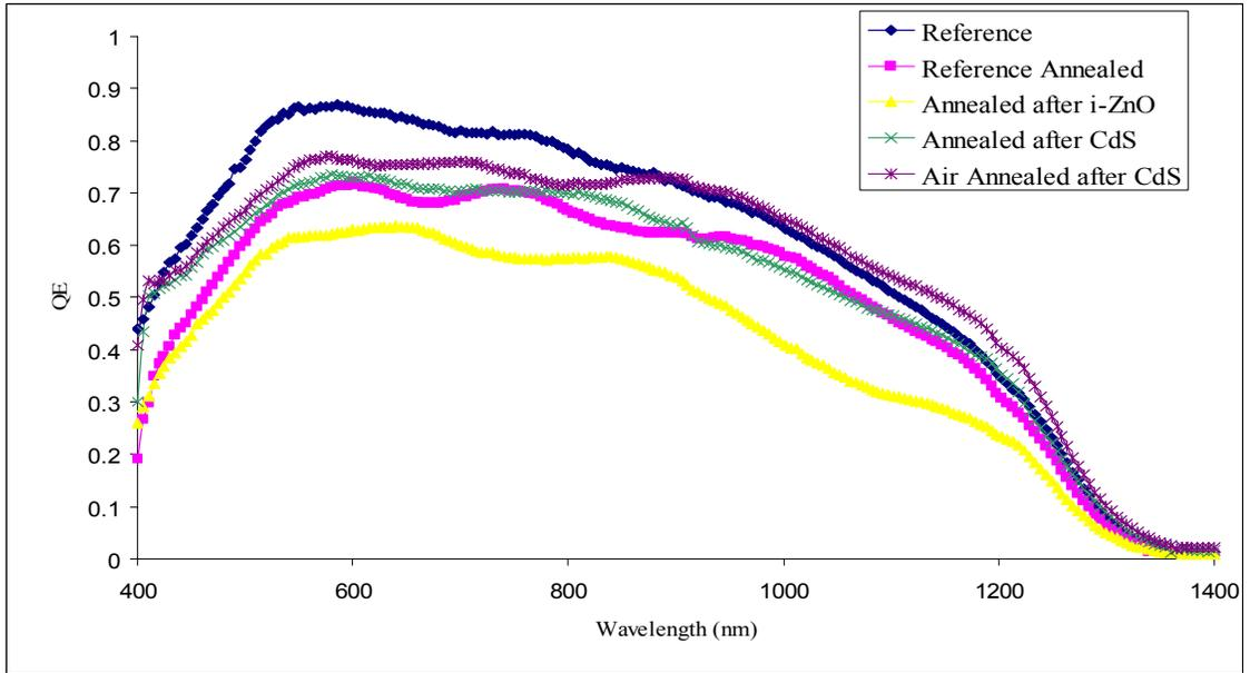
Figure 4.10: QE Profiles for Reference and Annealed Devices
