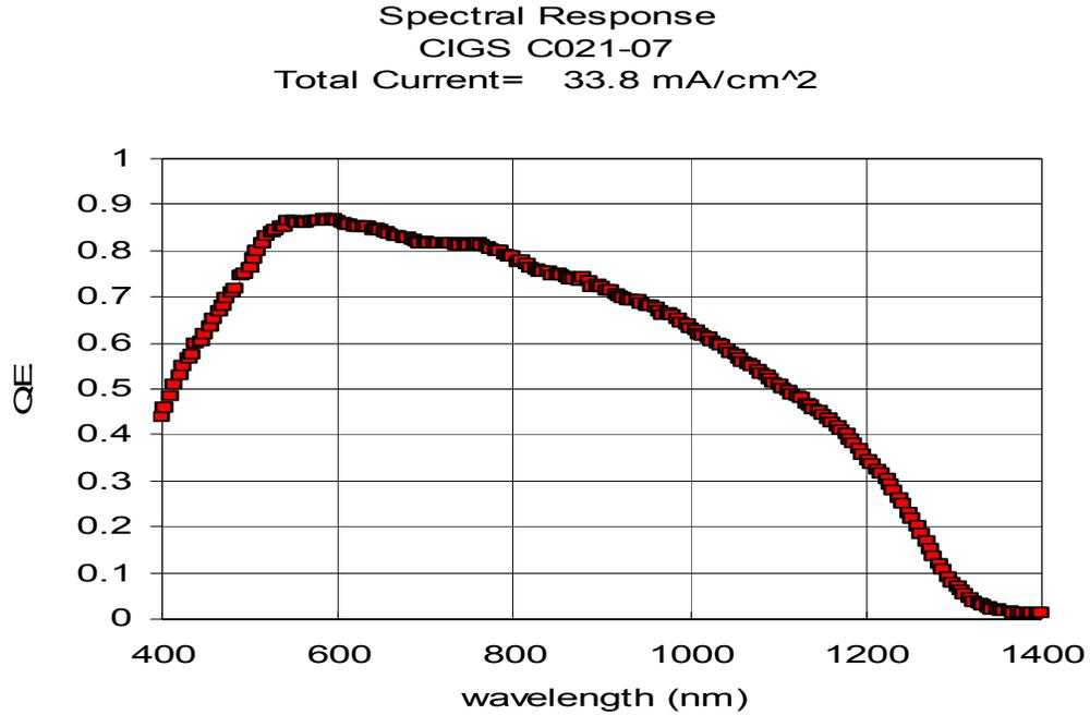
*Figure 4.7: Typical Spectral Response of a Standard Device*
