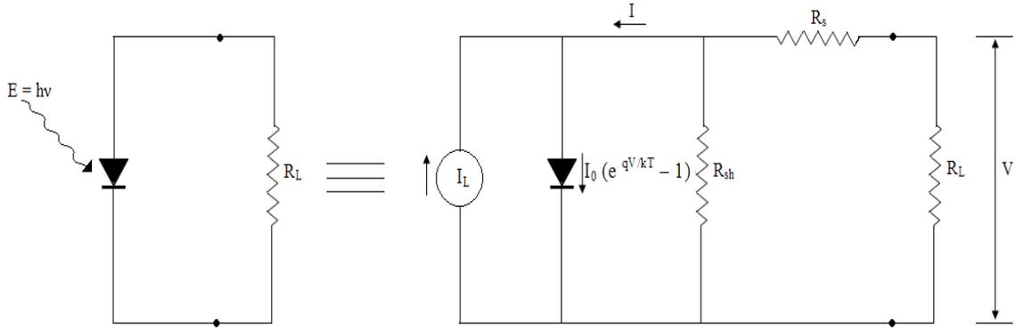
Figure 2.9: Equivalent Circuit of a Solar Cell
