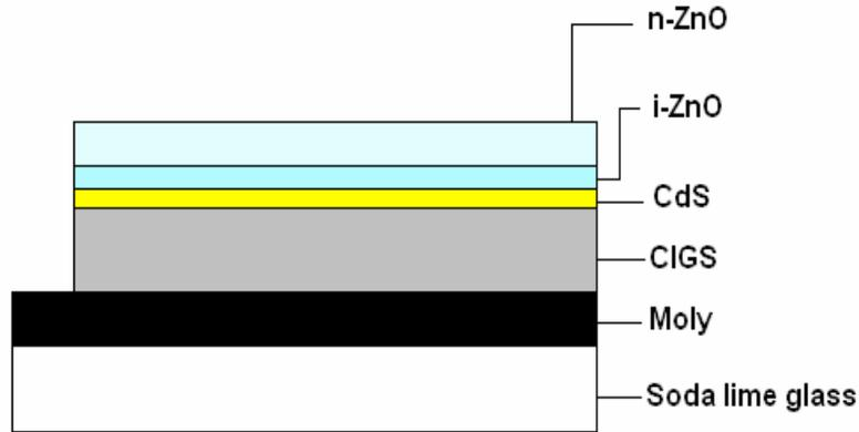
*Figure 3.2: Device Structure of CIGS Solar Cells*
