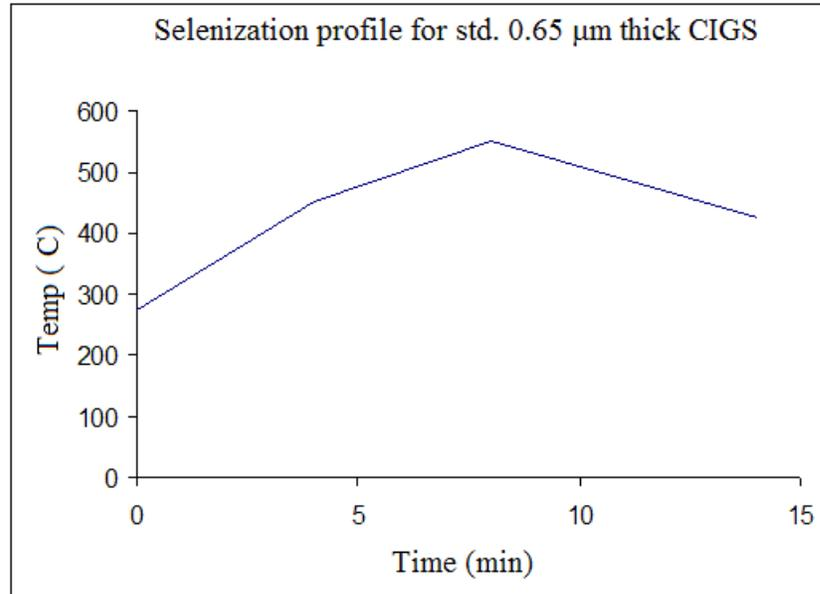
*Figure 3.6: Selenization Profile for std. 0.65 μm Thick CIGS*
