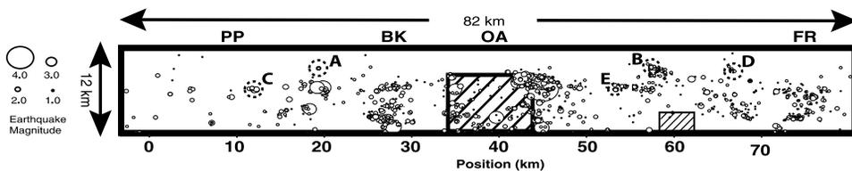
**Figure 2.** Fault-plane view of the Hayward fault, Model KT3 from Malservisi [2002] (see Figure 1 for location). Precisely-relocated micro-earthquakes from Waldhauser and Ellsworth [2002] are shown by circles scaled by magnitude. A through E mark several potential asperity locations (see text for details). Letters (PP, BK, OA, FR) correspond to locations from Figure 1.
