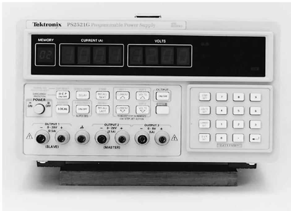
Figure 4.3: PS2520G Programmable Power Supply
