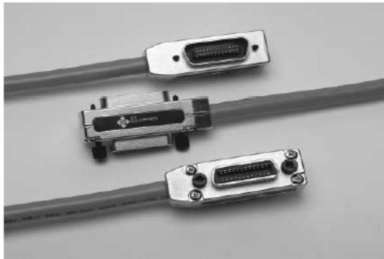
Figure 3.4: The GPIB IEEE-488 Connectors
