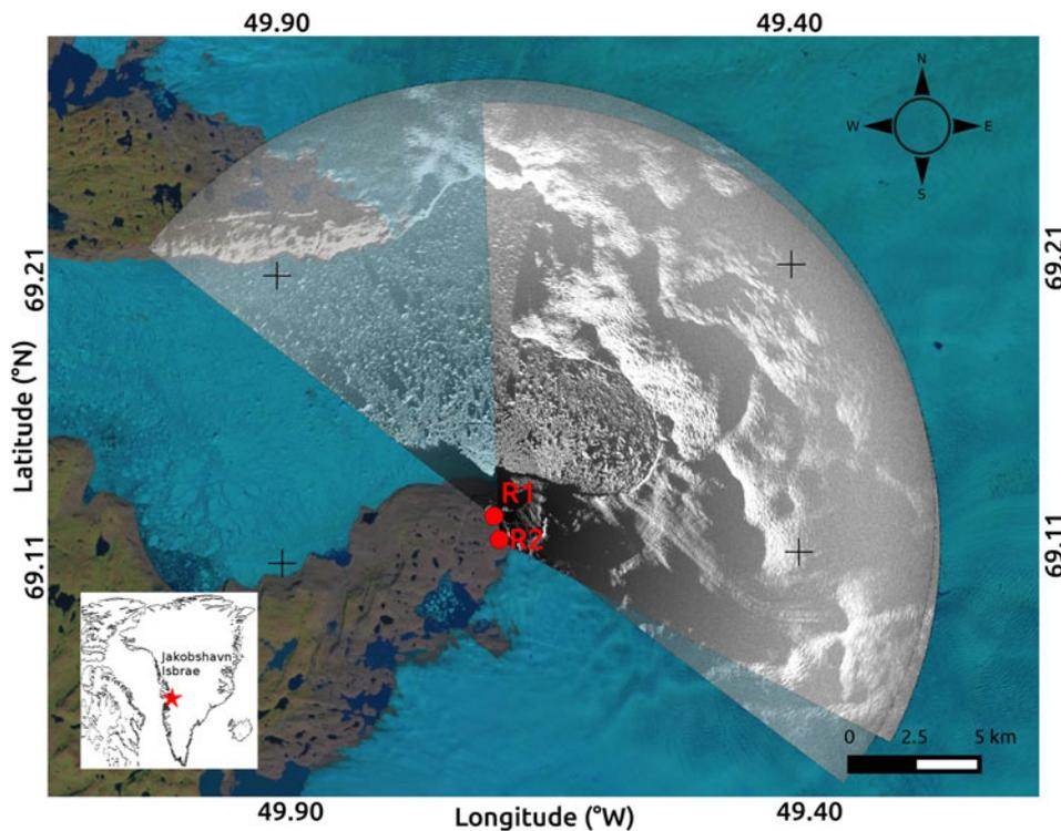
**Fig. 1.** Map of the field area. Site location relative to Greenland marked by red star (inset).  $R1$  and  $R2$  show the locations of the TRI instruments. Their respective coverage areas are shown by overlapping gray scales, overlain on a LANDSAT image from 11 August 2014 (obtained from landsatlook.usgs.gov).
