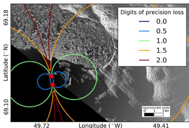
**Fig. 9.** Contours of loss of digits of precision considering the positions of the two radars (red stars) calculated from the condition number of the matrix of coefficients in Eqns (5) and (6). Most of the terminus experiences between 0.5 and 1.5 digits of loss.
