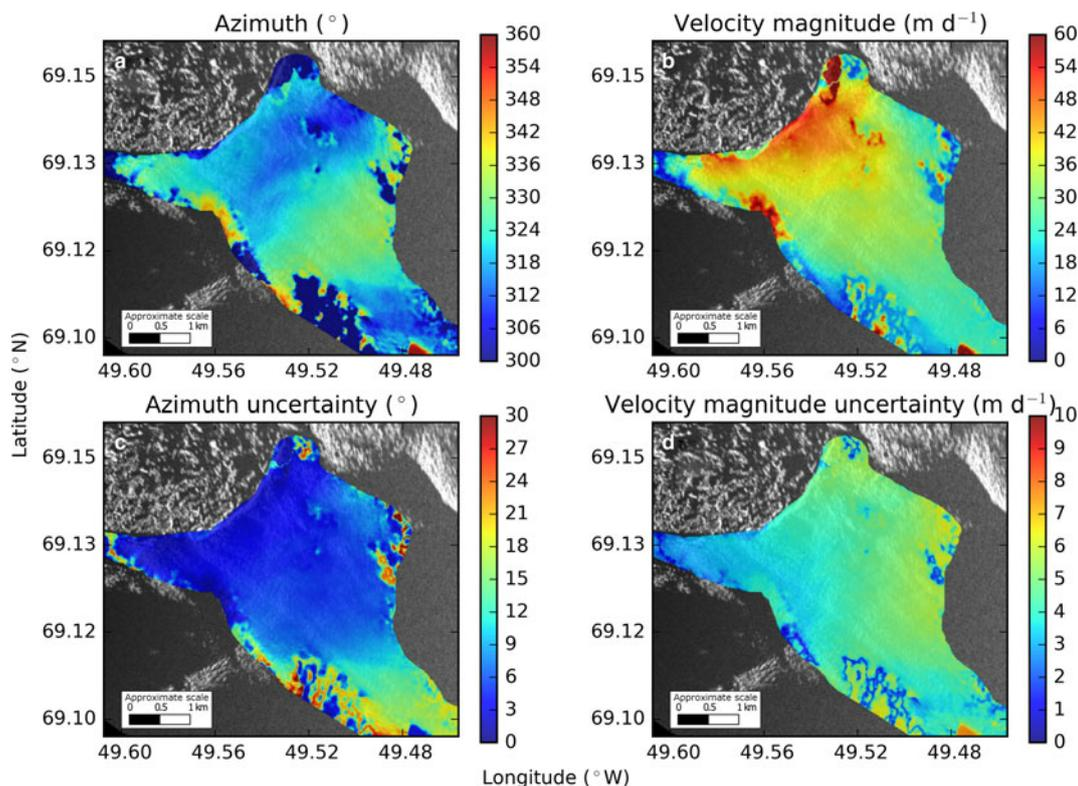
**Fig. 7.** Direction and velocity magnitudes derived from interferometry (a, b) and their respective uncertainties (c, d) are all calculated from the Monte Carlo simulation. Note that azimuth is defined to be positive clockwise from north.
