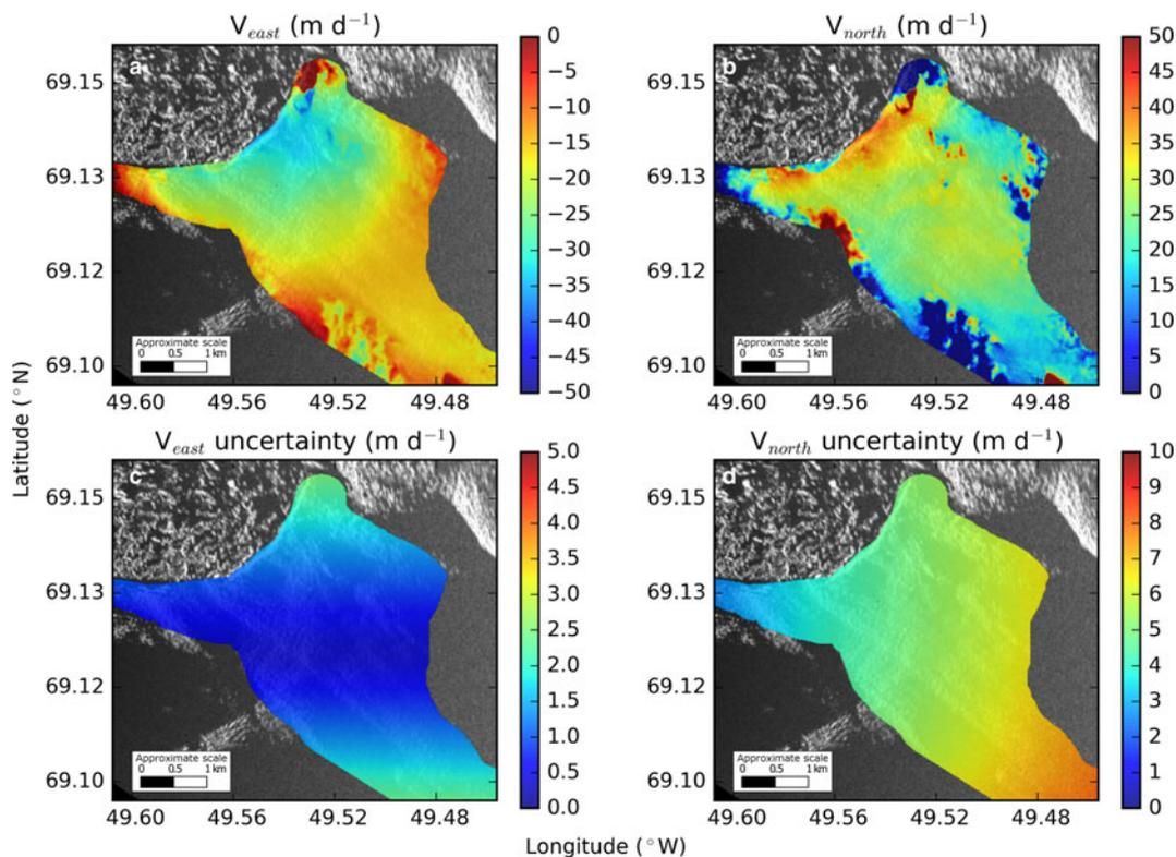
**Fig. 6.** East (a) and north (b) velocity component maps and their uncertainties derived from interferometry and the Monte Carlo simulation. Note that northward uncertainties (d) are higher than eastward uncertainties (c), likely due to the scan orientations of the two TRIs.
