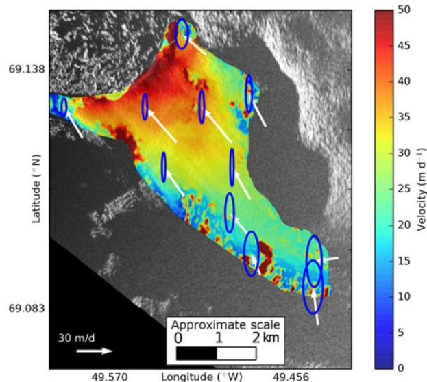
**Fig. 8.** Plot of error ellipses for a selected subset of points over the glacier surface overlain on a map of velocity magnitude derived from interferometry. The ellipses (blue) cover two SDs and are scaled relative to the arrows (white) showing the direction of motion and speed. Note that the north uncertainty is much greater than the east uncertainty.
