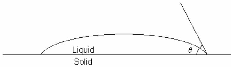
Figure 3: Diagram of the wetting angle  $\theta$
