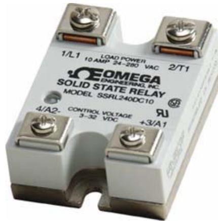
Figure 3.2: Solid State Relay (SSR)
