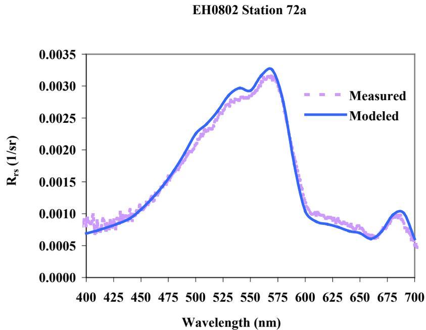
Figure 11. EH0802 Station 72a: Model Validation: Measured vs. modeled remote sensing reflectance.
