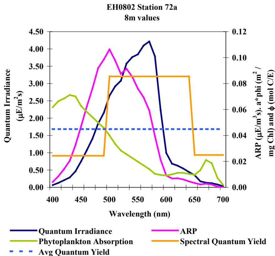
Figure 13. EH0802 Station 72a: Absorbed radiation by phytoplankton and its components (quantum irradiance and phytoplankton absorption) at 8m depth, compared against spectral and non-spectral quantum yield values for *Synechococcus* (adapted from Bidigare et al., 1989).
