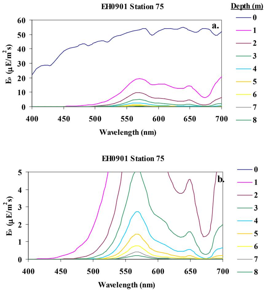
Figure 15. EH0901 Station 75: Quantum irradiance a.) from surface to bottom and b.) close-up of the bottom of the water column.
