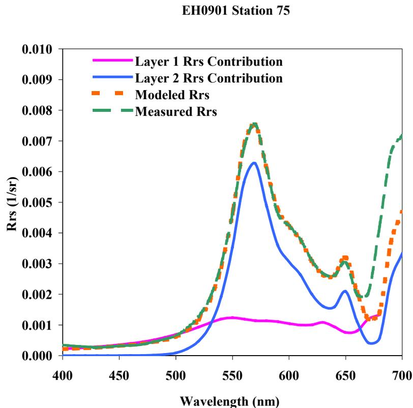
Figure 8. EH0901 Station 75: Model validation. Results of Lee’s optimization model using a two-layer system, compared against measured remote sensing reflectance at Station 75.
