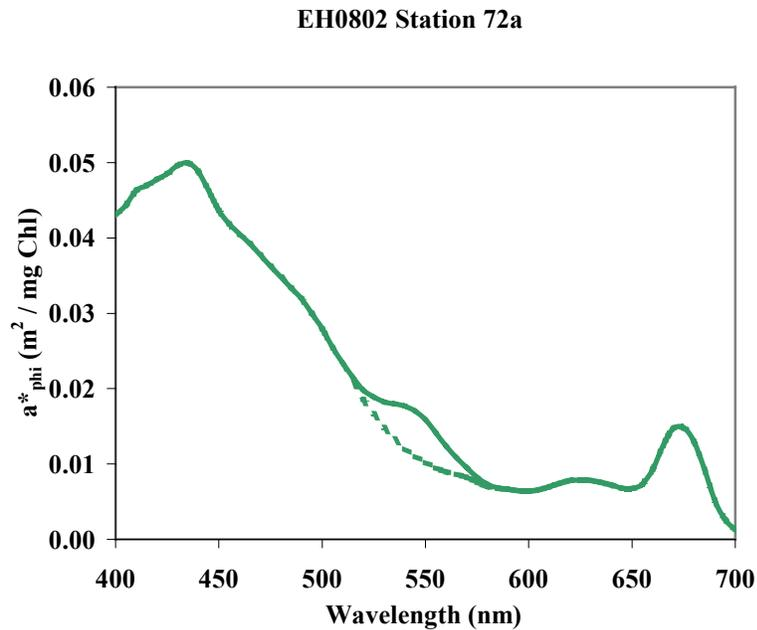
Figure 5. EH0802 Station 72a: Chlorophyll specific absorption curves for the phytoplankton component of the Hydrolight model. The dashed line shows  $a^*_{phi}$  with the 548 nm phycoerythrobilin peak removed.
