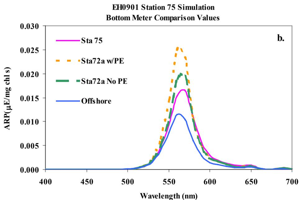
Figure 20. Comparison of absorbed radiation by phytoplankton at the bottom meter for various phytoplankton groups a.) below an upper layer with phytoplankton absorption with no phycoerythrin peak (“No PE”) b.) below an upper layer with phytoplankton absorption from the Station 75 *K. brevis* bloom. The same maximum and minimum quantum yield values are used for all simulations.
