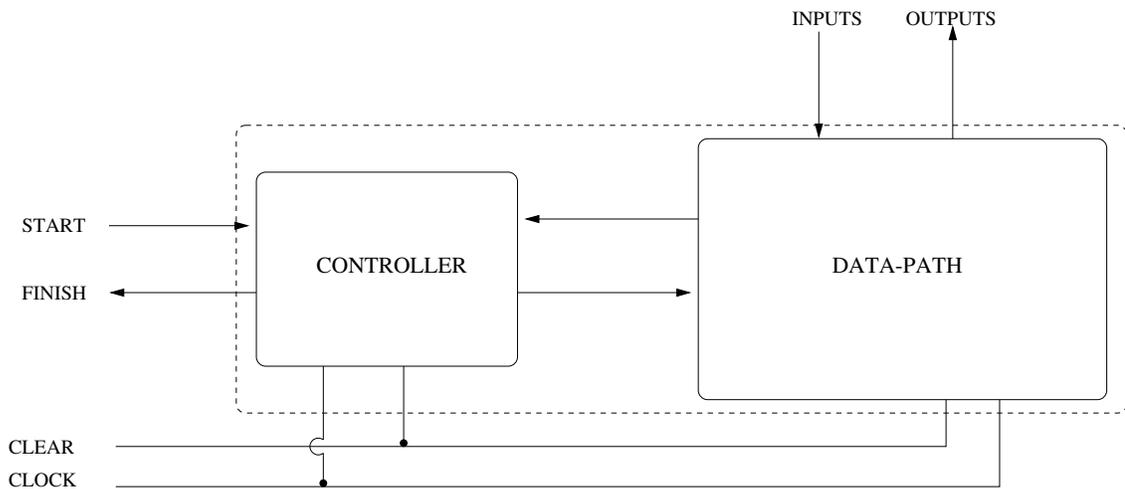
Figure 3.7. RT Level Design given by AUDI
