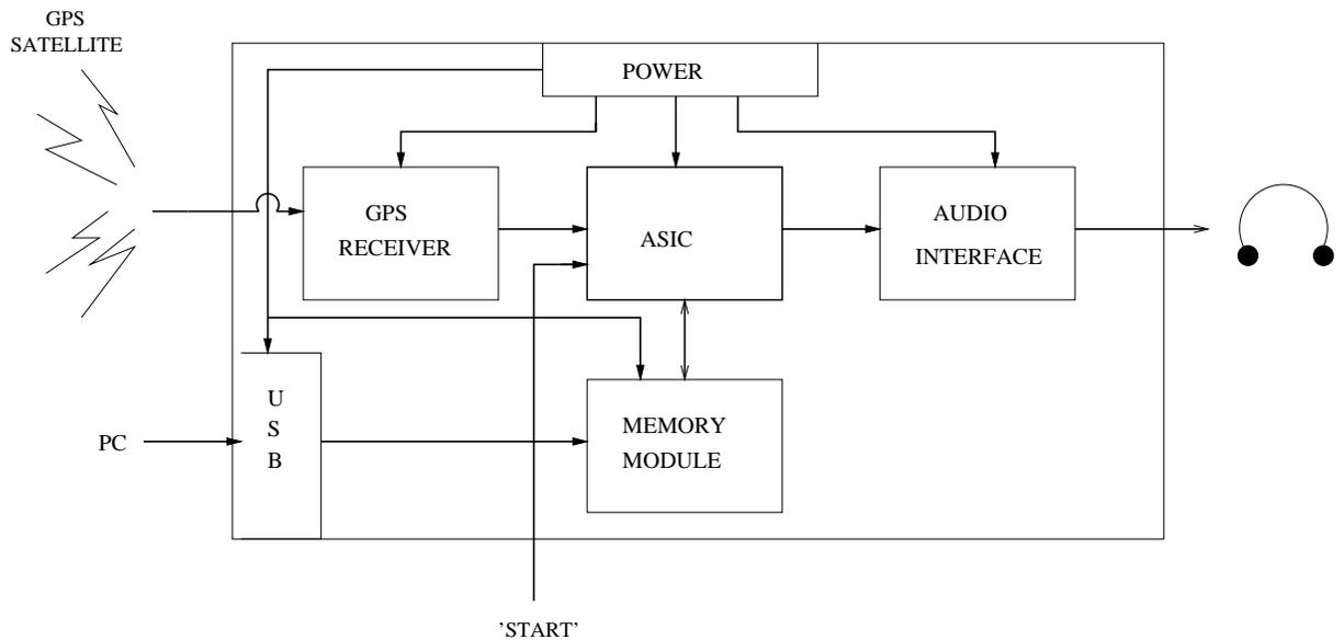
Figure 3.2. Overall Block Diagram of the System Design
