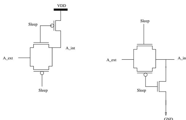
Figure 2.15. Modified Latches with Optimum Sleep Values (0 and 1)
