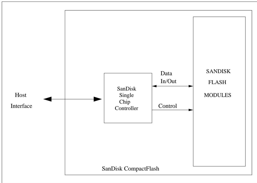
Figure 3.3. Compact Flash Memory Card Block Diagram
