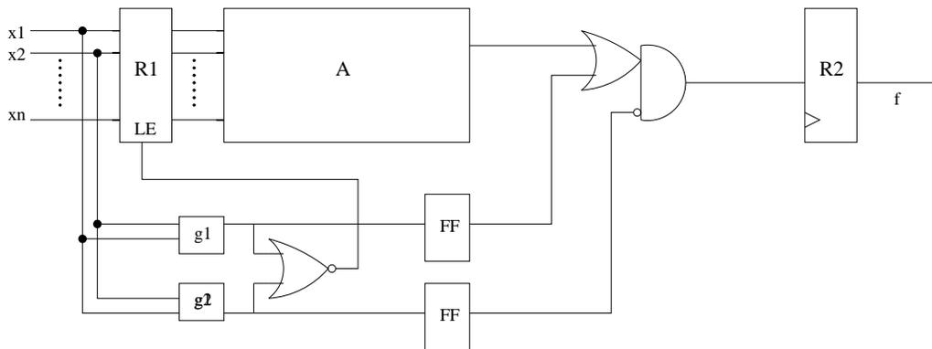
Figure 2.6. First Precomputation Architecture
