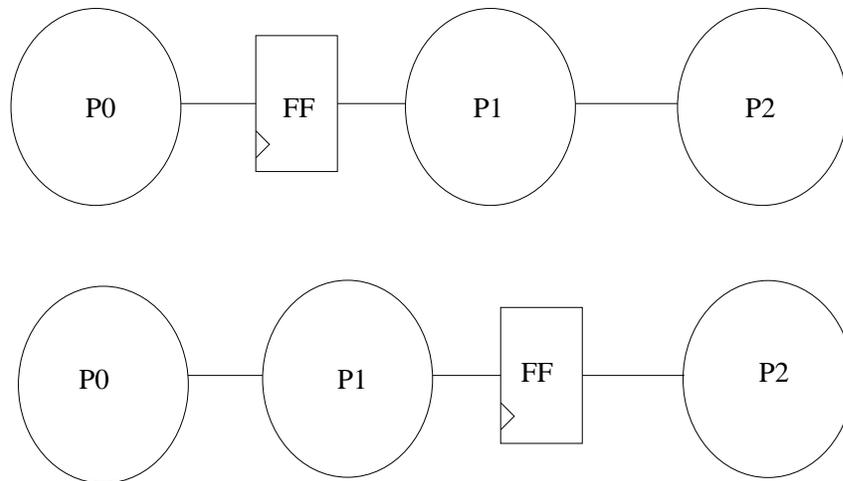
Figure 2.11. Repositioning the Flip-flops in a Pipeline
