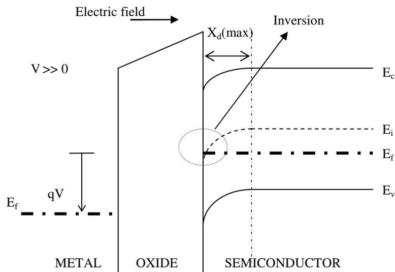
**Figure 2.4** Band Diagram of MOS at a Large Positive Voltage
