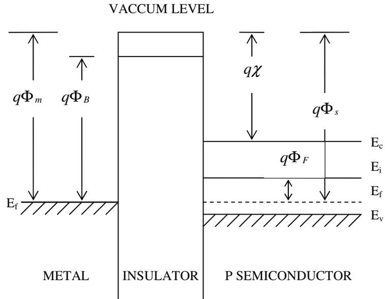
**Figure 2.1** Band Diagram for Ideal MOS Diode [10, 11]
