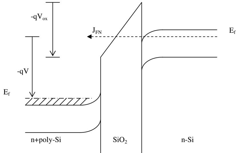
**Figure 3.2** Energy Band Diagram for an n+poly-Si/SiO<sub>2</sub>/n-Si Structure in Case of Fowler Nordheim Tunneling
