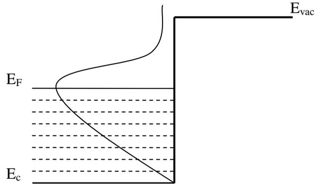
**Figure 3.1** Thermionic Emission
