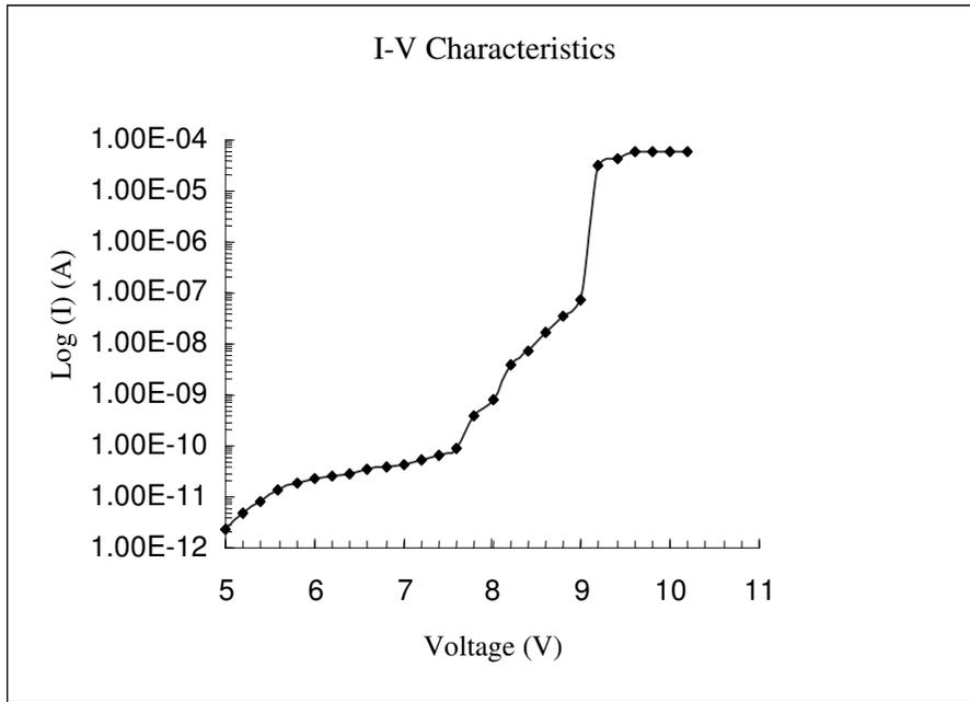
**Figure 4.10** I-V Characteristic for a 7 nm p-type Device
