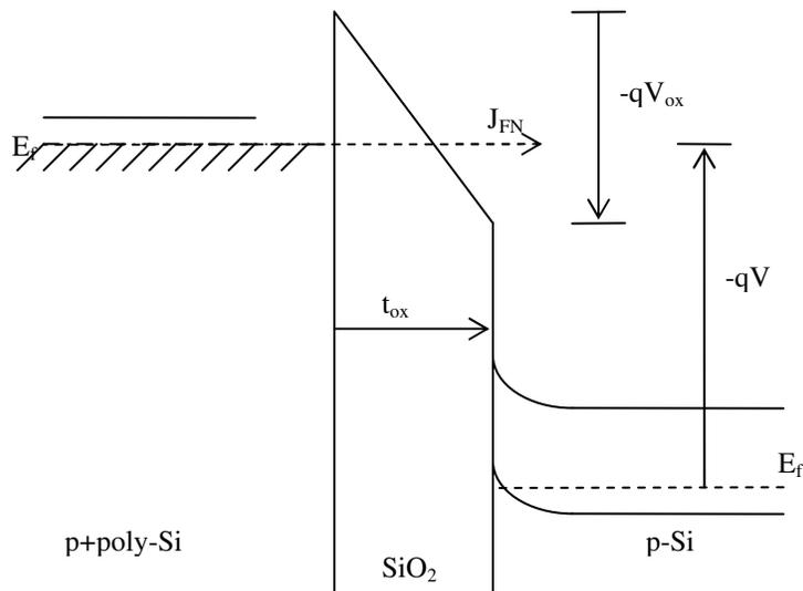
**Figure 3.3** Energy Band Diagram for a p+poly-Si/SiO<sub>2</sub>/p-Si Structure in Case of Fowler Nordheim Tunneling
