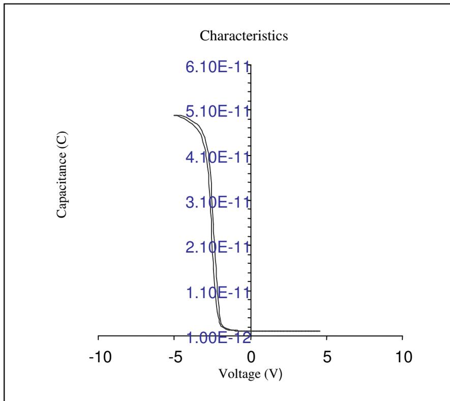
**Figure 4.8** C-V Characteristics of a 7 nm p-type Device
