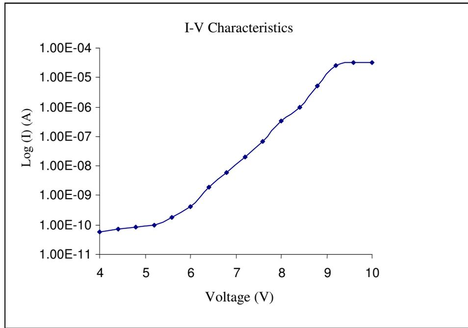
**Figure 4.9** I-V Characteristic for a 7 nm n-type Device
