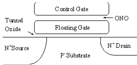
**Figure 2.14** Basic Structure of a Typical FG Device
