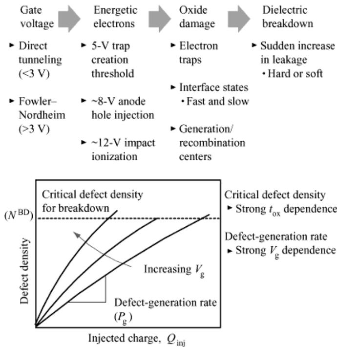
**Figure 3.6** Outline of the Mechanism of Defect Generation Leading to Breakdown of SiO<sub>2</sub> [26]
