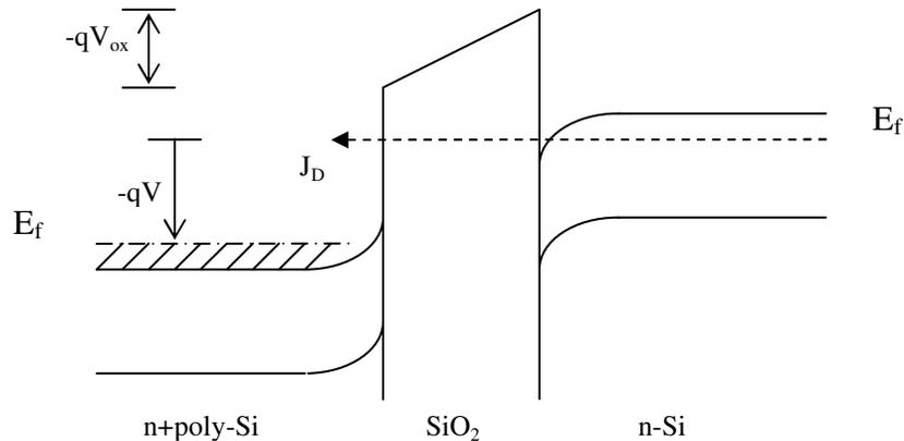
**Figure 3.4** Energy Band Diagram for an n+poly-Si/SiO<sub>2</sub>/n-Si Structure in Case of Direct Tunneling
