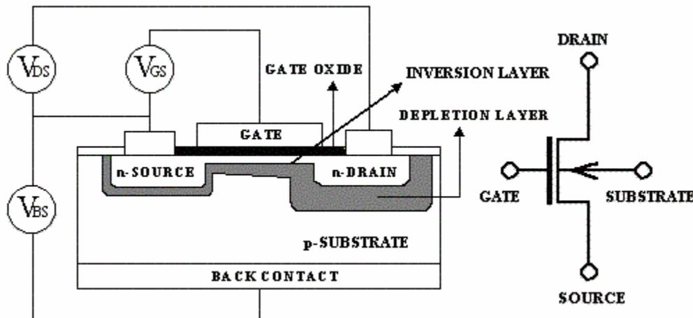
**Figure 2.11** Cross-Section and Circuit Symbol of an n-channel (MOSFET)
