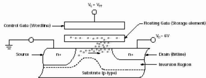
**Figure 2.15** Flash Cell During a Write Operation [16]
