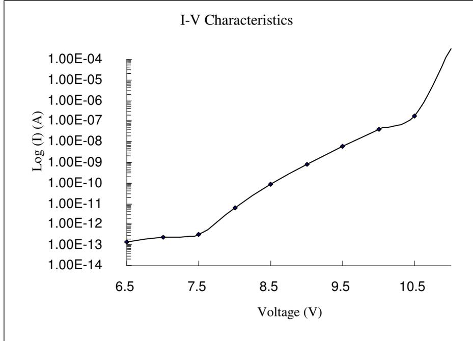
**Figure 4.12** I-V Characteristic for a 10 nm p-type Device
