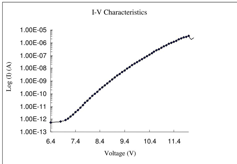
**Figure 4.11** I-V Characteristic for a 13 nm n-type Device
