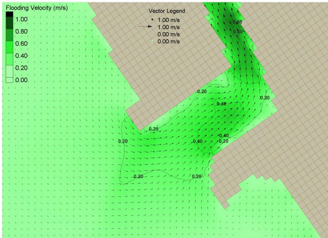
Fig. 8. Examples of modeled ebb (upper panel) and flood (lower panel) flow patterns through Blind Pass.
