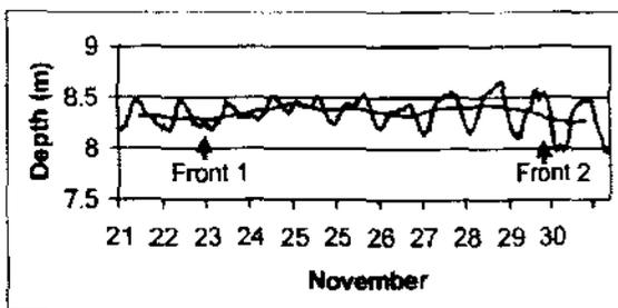
Fig. 5. Hourly water level and water level smoothed using a 24-h moving-average window.
