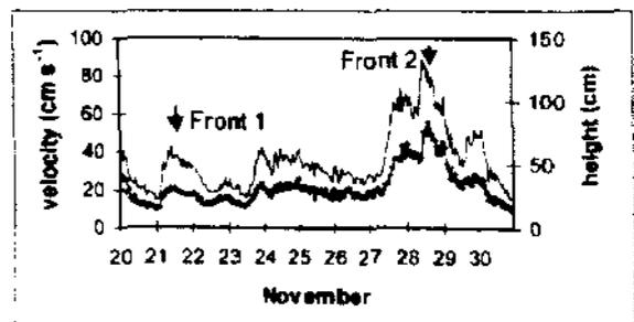
Fig. 4. Significant wave height (smooth line) and wave orbital velocity (marked line) during the study period.
