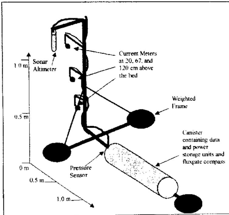
Fig. 2. Schematic diagram of the WADMAS instrumentation system.
