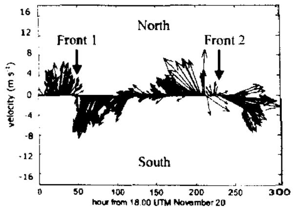
Fig. 3. Hourly wind velocity vectors (m s<sup>-1</sup>). Arrows indicate the direction in which the wind was blowing (oceanographic convention).
