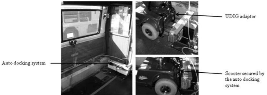
**Figure 3. Auto docking system installed in LATV (left); scooter equipped with UDIG adaptor, backed into and secured by auto docking system**
