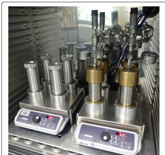
**Figure 1 High-pressure reactors and control reactors.** High-pressure reactors (right, made from stainless steel and bronze, max. pressure 40 MPa, pressurizing with N<sub>2</sub> gas, 160 mL volume) and aluminum control reactors (left, max. 0.1 MPa, 160 mL volume) were used for cultivation of hydrocarbon degraders at high and ambient pressure. The cultures were mixed with magnetic stirrers.
