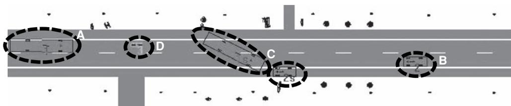
Note: A: Initial position of bus, B: Initial position of pickup truck, C: Point of rest, D: Initial position of motorcycle.
