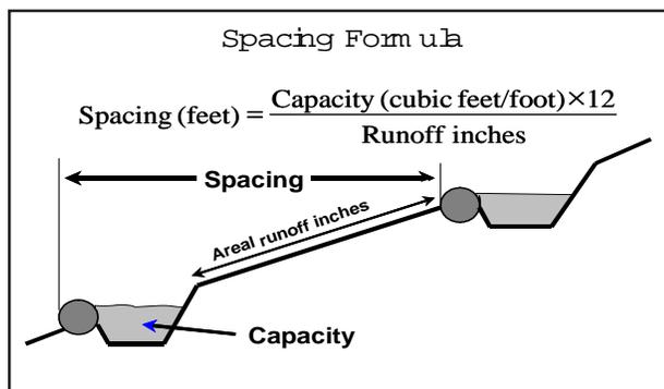
Figure 2. Spacing formula for contour basin design.
