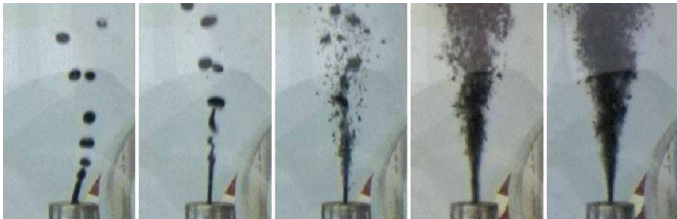
FIGURE 1. Oil droplets discharged into water through a 2 mm diameter nozzle (Tang and Masutani, 2003). From left to right, the jet exit velocities are 0.31, 0.97, 1.41, 2.42, and 5.99 m s -1 . As a point of reference, the nozzle outer diameter is 2.5 cm.
