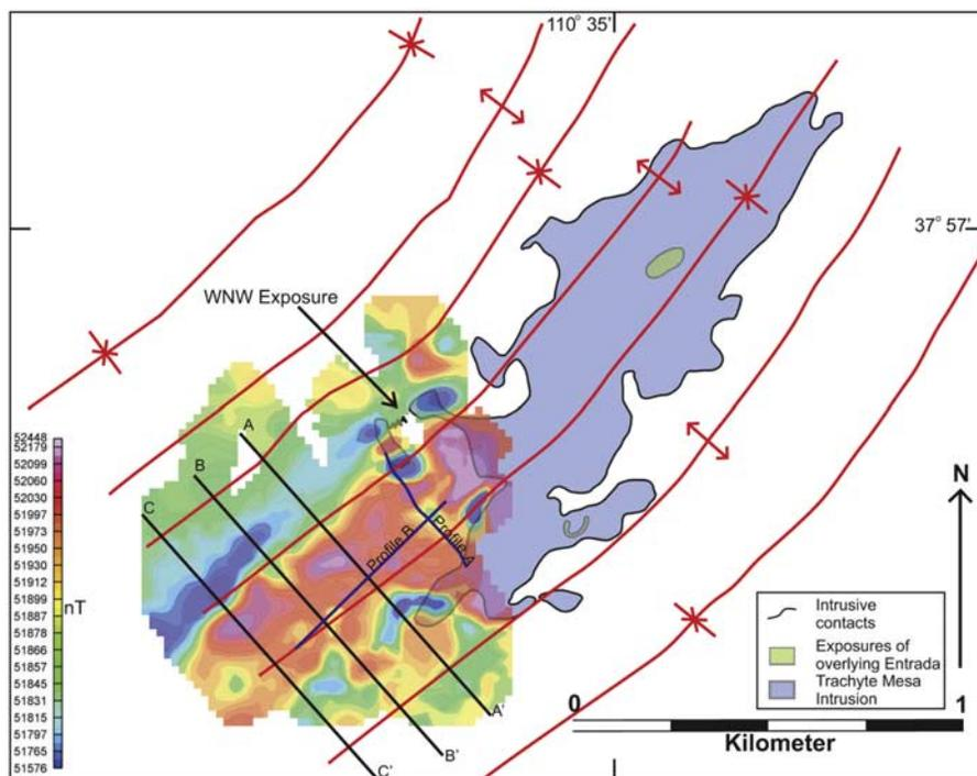
**Figure 3.** Map of the Trachyte Mesa intrusion including fold traces with the magnetic map overlain. Heavy purple lines show the locations of the resistivity experiments. Magnetic map shown as anomaly in the total magnetic field (nanoteslas). Lines A–A', B–B', and C–C' correspond to the magnetic models shown in Figure 4. Magnetic and resistivity data can be obtained from the authors upon request.
