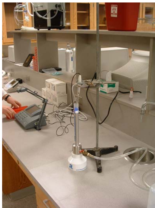
Figure 5: Measurement of pH of Breath Condensate While Undergoing Deaeration with Argon Gas
