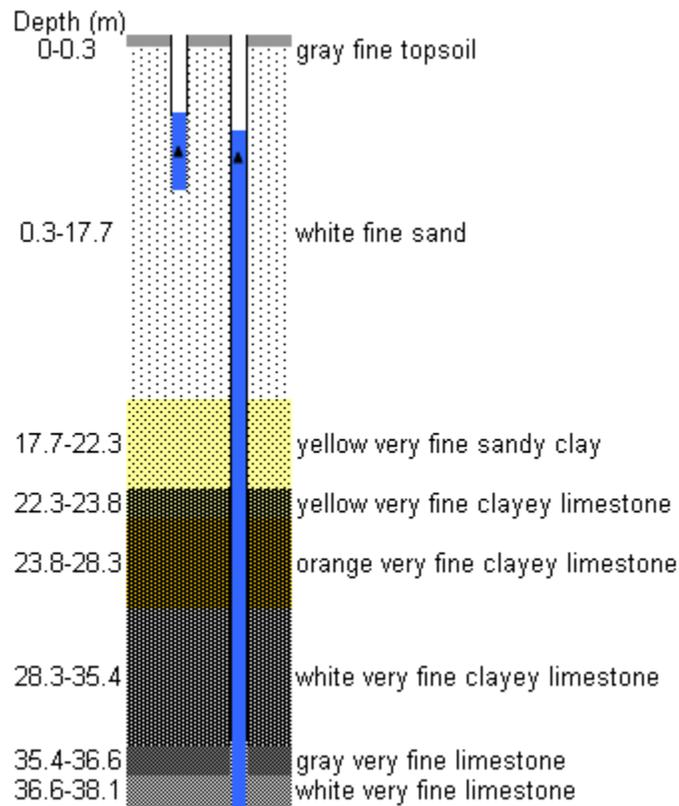
Figure 7 Soil layers and well depths (cross-section) at Site 4.
