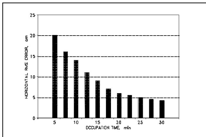
**Figure 2.** Performance of the Trimble Phase Processor v.2 software with the GPS Pathfinder PRO XR system according to Trimble (1997). Figure modified from Trimble (1997). Horizontal errors are shown; however, Trimble (1997) states that vertical and horizontal errors are similar for phase processed solutions.
