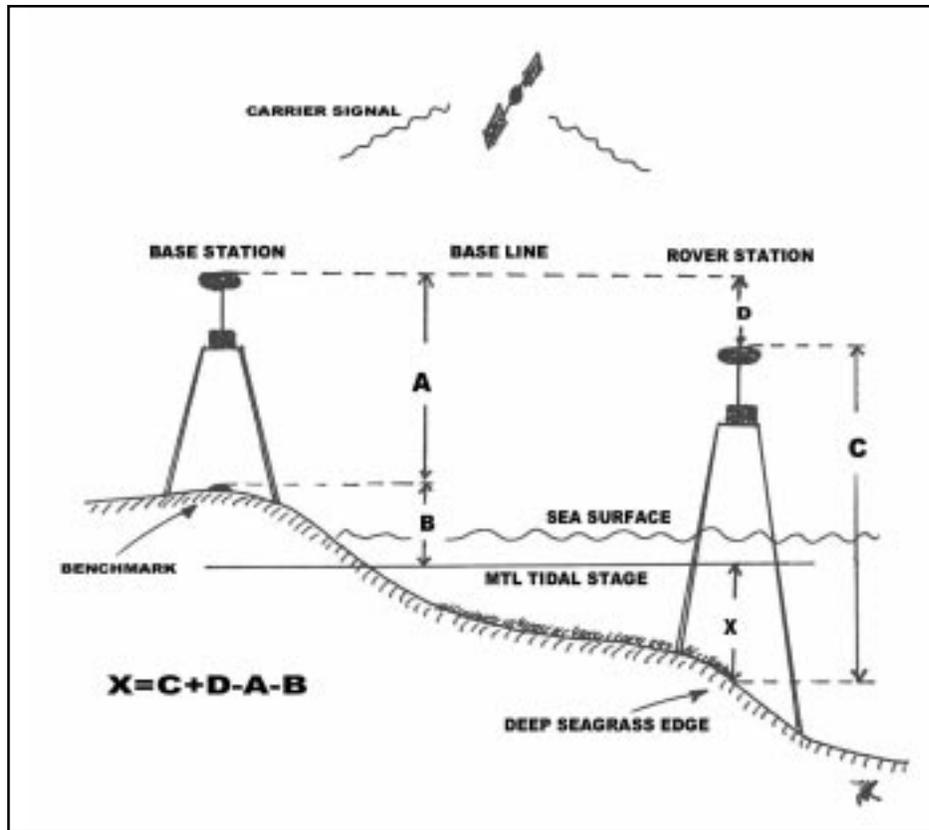
**Figure 6.** Schematic of typical GPS stations set-up during elevation measurements. A = base station antenna height; B = benchmark elevation above MTL tidal stage; C = rover station antenna height; D = Relative elevation difference between base station and rover station antennas; X = Calculated elevation of the deep seagrass edge.
