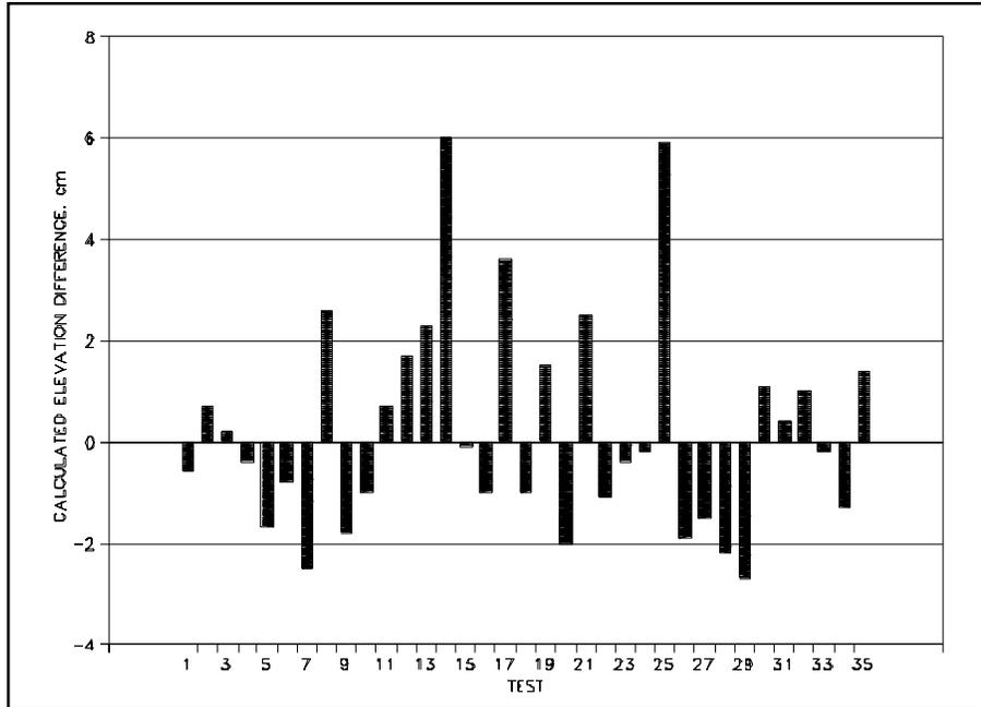
**Figure 8.** Results from 35 tests of vertical measurement errors conducted on the roof of the City of Tampa Bay Study Group laboratory using two Pathfinder PRO XR instruments. The true elevation difference between the instruments was 0 cm.
